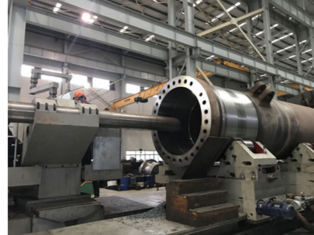
DEEP HOLE BORING
